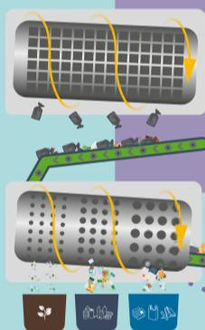
First our mechanical treatment technology sorts and separates the waste. An amazing 1.5km of conveyor belts move the waste between a range of sorting techniques, including magnets, sifting, trommels (large drum shaped sieves) and infra-red detectors. We take out anything that's recyclable, such as plastic and cans. We also take out organic waste like food and garden materials.
